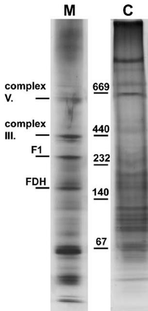
Fig. 3. Native polyacrylamide gel electrophoresis of mitochondrial and cytoplasmic protein complexes (see Section 2.7). M: mitochondrial fraction; C: cytoplasmic fraction; F1–F1-ATPase; FDH: formate dehydrogenase; the numbers refer to the size of standard protein complexes (669 kDa: thyroglobulin; 440 kDa: ferritin; 232 kDa: catalase; 140 kDa: lactate dehydrogenase; 67 kDa: bovine serum albumin).
