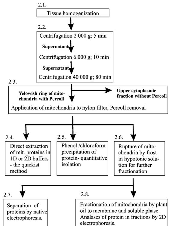
Fig. 2. Scheme for the isolation and sub-fractionation of mitochondria. Boxed labels correspond to sections as described in Section 2.
