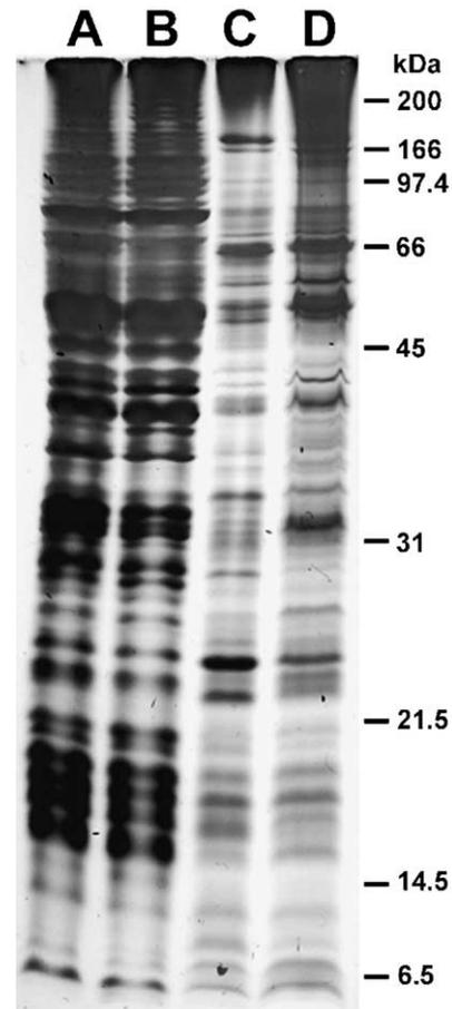
Fig. 4. 1-D SDS-PAGE of protein fractions obtained during isolation of mitochondria from in vitro cultivated pollen. A: crude homogenate; B: cytoplasmic fraction (supernatant; see Sections 2.2 and 2.3); C: mitochondrial fraction separated by Percoll and trapped on nylon filter (see Sections 2.2 and 2.3); D: mitochondrial matrix fraction after sunflower oil sub-fractionation (see Section 2.8).
