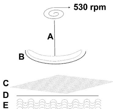
Fig. 1. Schematic representation of the blender used for plant tissue homogenization. The rotary part consisted of a piston (A) with attached 1 mm nylon mesh (B). The stationary part consisted of a  $45\ \mu\text{m}$  nylon mesh (C) and Saran foil (D) attached to the soft support (E).
